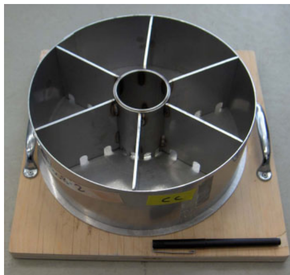
Fig. 1. Six-chambered, stainless-steel earthworm avoidance test unit. Alternate chambers are filled with treatment and control soils. Earthworms move from the central cavity to one of the peripheral chambers and are then free to move between these chambers. External ring diameter measured 240 mm; internal ring diameter measured 60 mm. [Color figure can be seen in the online version of this article, available at wileyonlinelibrary.com ]
